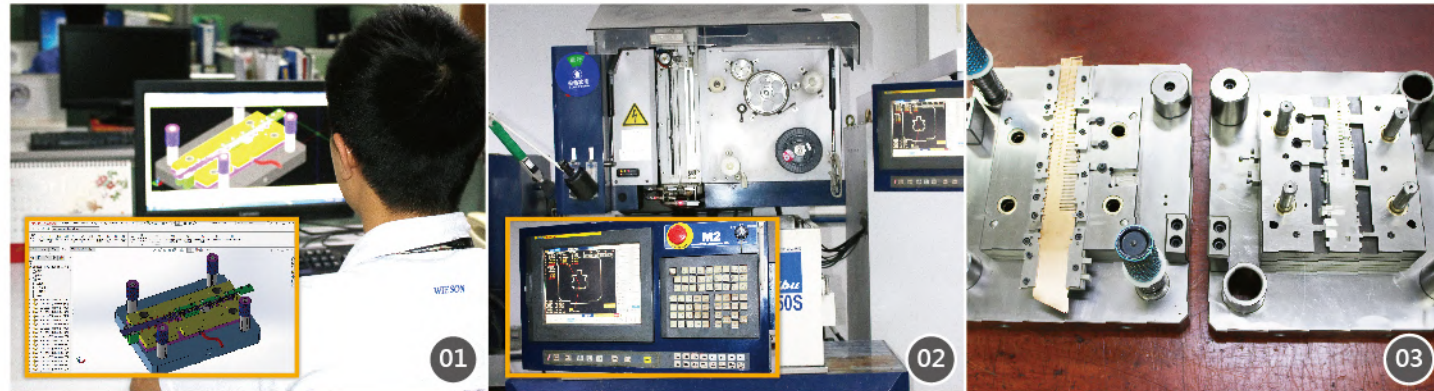
01 Hardware Mould 3D Design (3D Simulated Forming) 五金模具3D設計(可3D模擬成型) 02 Precision Slow-Walking Wire Processing (Machining Accuracy up to 2u) 精密慢走絲加工(加工精度高達2u) 03 Precision Hardware Mould (Stamping Material Thickness 0.1mm~1.6mm) 精密五金模具(沖壓料厚0.1mm~1.6mm)
