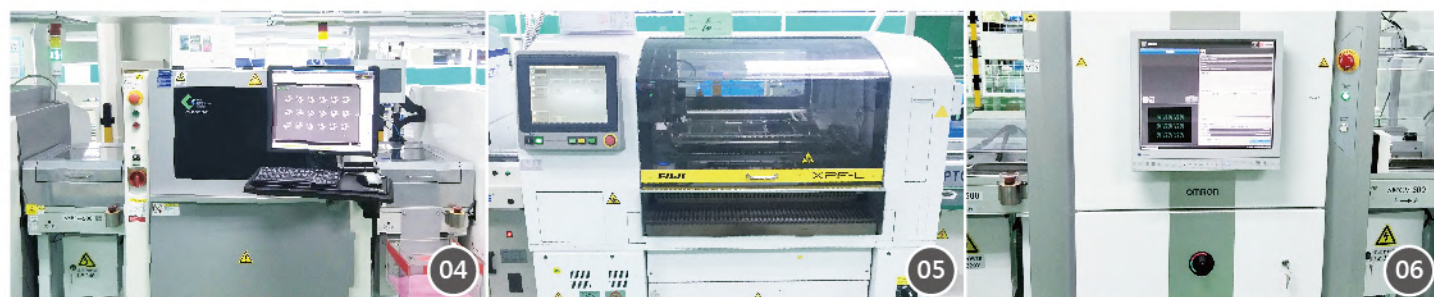
Auto Solder Paste Thickness Machine(K8030-2) Highly repetitive: ±2% 全自動錫膏測厚機(K8030-2) 高度重複性: ±2%
