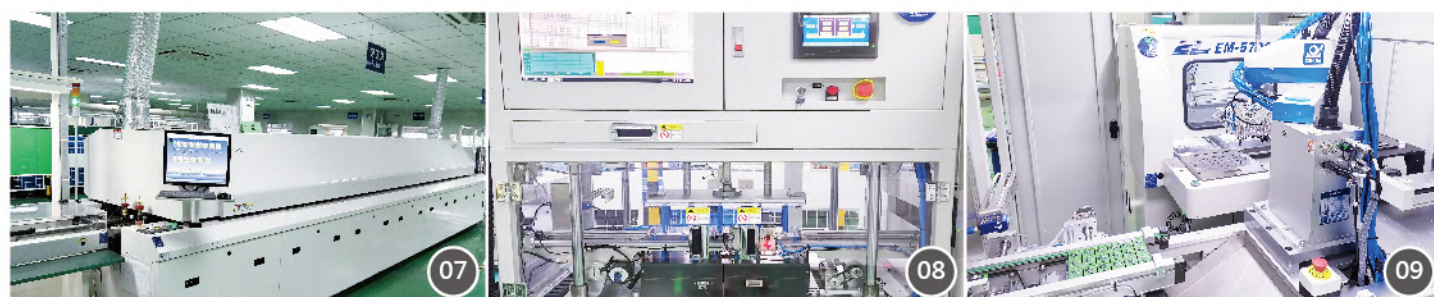
Lead-Free Nitrogen Reflow Soldering(JTR-1200) Temp. control precision: ±1.0°C, can satisfy the patch, plug-in, spraying, etc 無鉛氮氣回流焊(JTR-1200) 溫度控制精度: ±1.0°C, 可滿足貼片、外掛程式、噴塗等工藝
