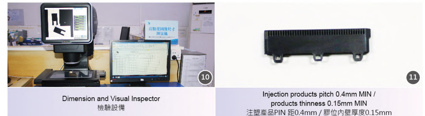
10 Dimension and Visual Inspector 檢驗設備 11 Injection products pitch 0.4mm MIN / products thinness 0.15mm MIN 注塑產品PIN 距0.4mm / 膠位內壁厚0.15mm
